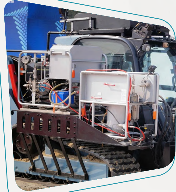
Unexploded Ordnance Handling Robot (UXOR), an advanced Unmanned Ground Vehicle (UGV) Photo: DefenceXP
